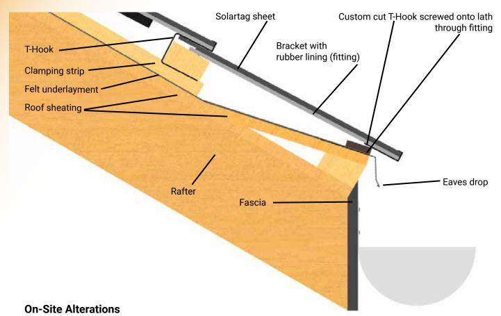
The first T-Hooks (entire row by the gutter) is adapted with an angle grinder, by taking off the back part of the clamp. This allows the T-Hook to be screwed to the lath. Note that the first row of brackets are screwed onto the first lath by drilling through the aluminium railing under the rubber.
