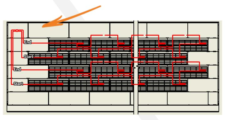
When the first active sheet is laid, you also place a cord from the sheet to the location, where you intend to place the inverter (stater cord). This cord must be taped at the end - because solar cells always produce electricity - and you risk jolts.
