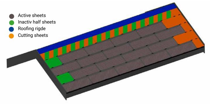
**NOTE:** The model above is a simple roof solution. If the roof is adapted to Solartag's dimensions, active sheets can be used all the way up to roofing ridge as well on the closing side.
